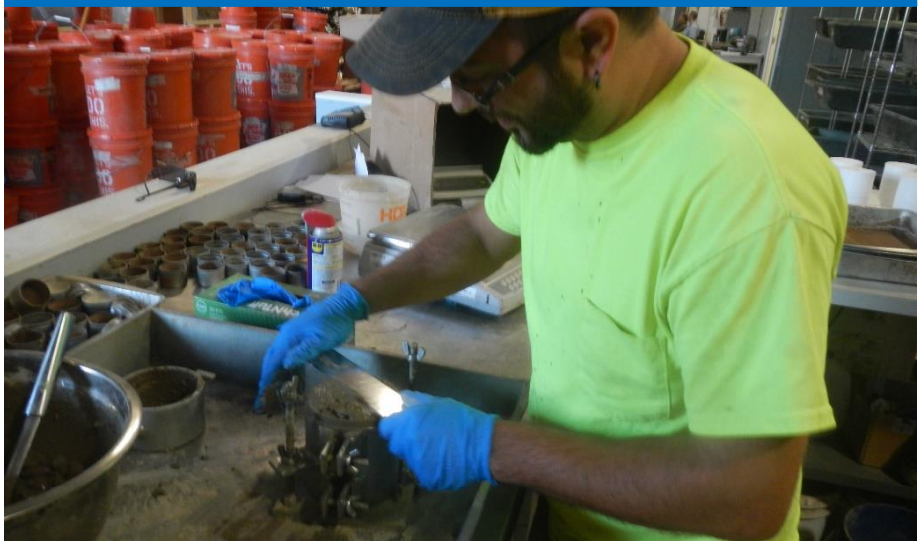
Photos demonstrate Stahl Sheaffer's FDR with proctor tests completed for the project at Stahl Sheaffer's Soils & Materials Lab.
