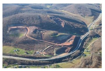
The New Baltimore landslide, located along the Pennsylvania Turnpike in Somerset County, has been problematic for the Turnpike ever since its construction in 1939. Being an active landslide, it continues to move toward the eastbound lane at a rate of approximately 6-10 inches/year causing the shoulder and right lane to heave approximately 8 inches/year. Overall, this ancient landslide is a translational failure with localized rotational slides, rock falls, and flows.
